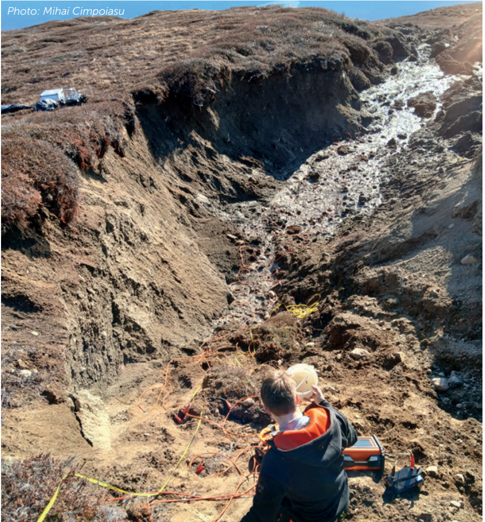
Anton Abrahamsen seen here setting up the geophysical survey line along the mudslide.
